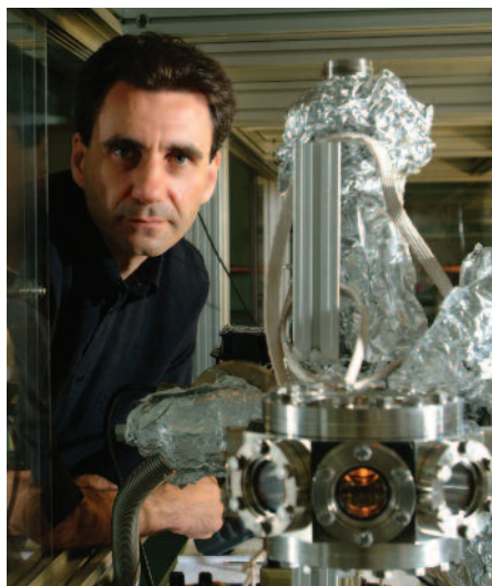
Dr. Ron Folman next to a vacuum chamber where atoms are isolated, as required for quantum features to dominate their behavior
