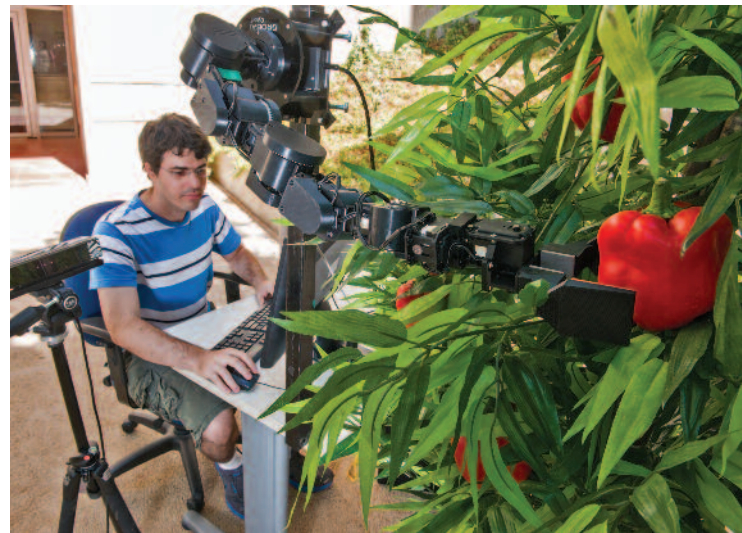
Ph.D student Efi Vitzrabin with a robot that detects the ripeness of crops, such as a pepper, and picks it from the plant without damaging the crop.
