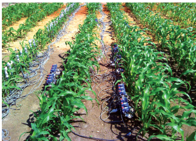
Monitoring soil variability with tensiometers, which measure moisture and irrigation needs
